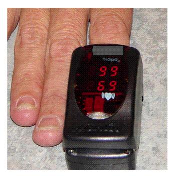
Fig 1. Pulse oximeter—placement on right index finger.
